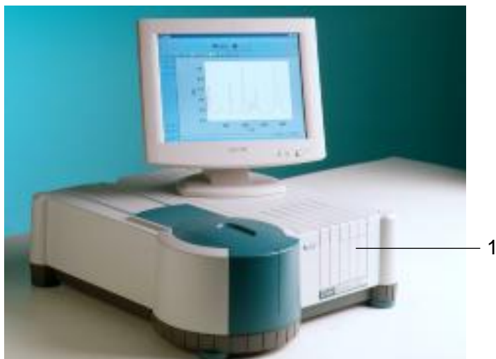
Figure 5. The snap-out panel (1) on the front of the Cary 50
